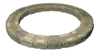
**3.** Build the bottom layer by laying 23 8" tapered caps in a circle. You may have to adjust the blocks and use a rubber mallet to get the blocks to fit.
