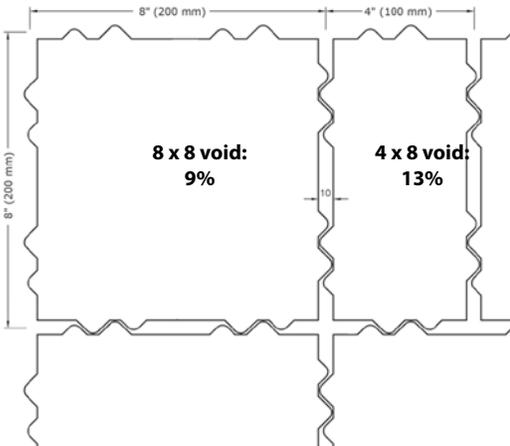
When building permeable pavement structures with Eco-Priora 4 x 8 or 8 x 8, follow design and construction recommendations found in "Permeable Interlocking Concrete Pavements- 4th Edition" as published by the Interlocking Concrete Pavement Institute (ICPI, 2011). Copies are available from ICPI ([www.ICPI.org](http://www.ICPI.org)) or your Mutual Materials representative.
