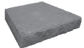
Split Face Tapered Cap Unit 18" (front face) 12" (back face) x 3" x 13" (45.7 cm x 7.6 cm x 33 cm)
